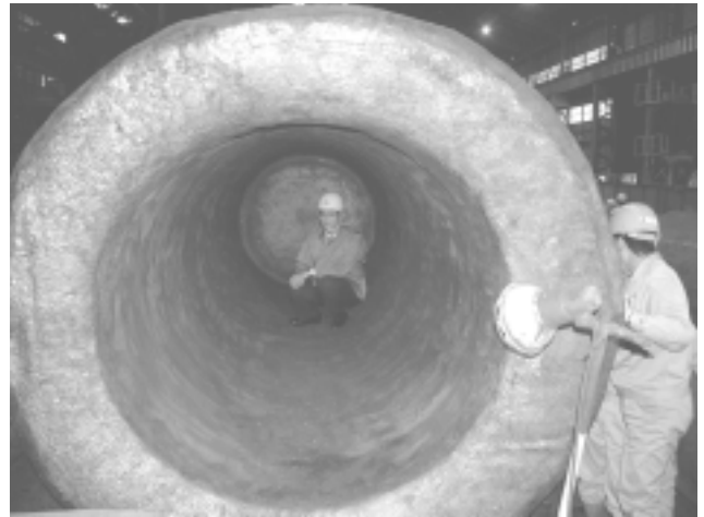
Fig.2 Forged steel for MSF series cask
