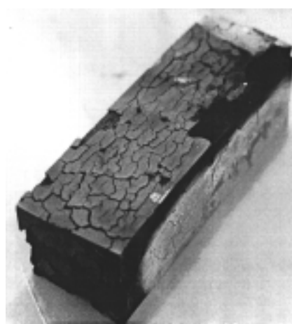
Fig.10 Photograph of test piece after fire test
