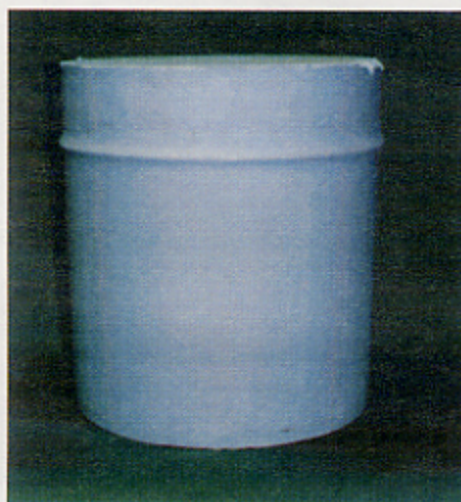
Fig.4 Waste form made of new cement with 20L volume
