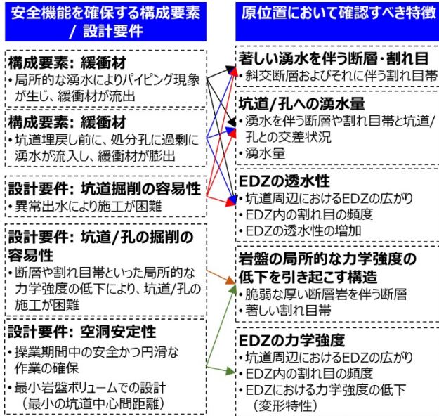
Fig. 6 Relationship between the components/design requirements to ensure the safety functions targeted in Task B and the features to be identified in the in situ investigation.
