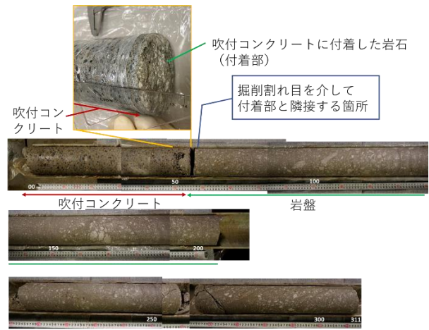
Fig.5 \Phi 116 \text{ mm} samples for SEM observation, extracted ions and density measurements, and permeability test.
