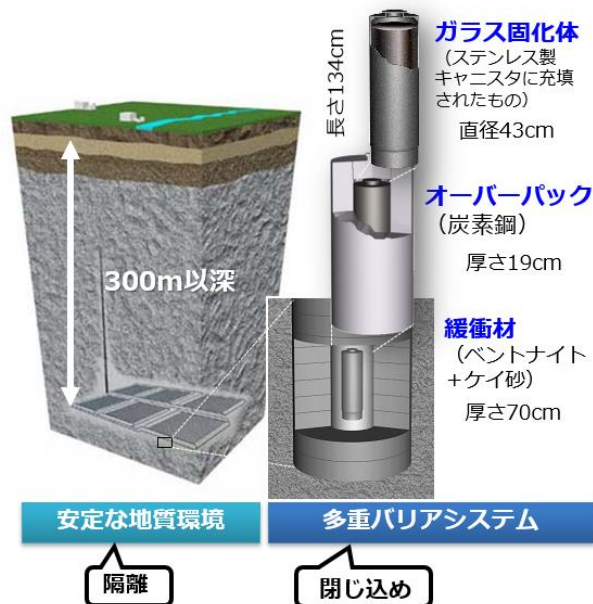
Fig.1 Basic concept of geological disposal system [2]
