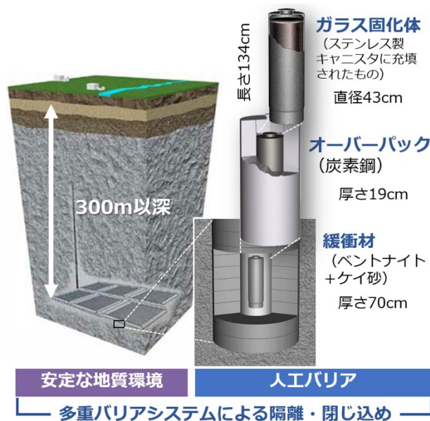
Fig.1 Basic concept of geological disposal system
