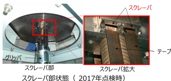
Fig.21 Parts of gripper drive mechanism that may cause sliding resistance
