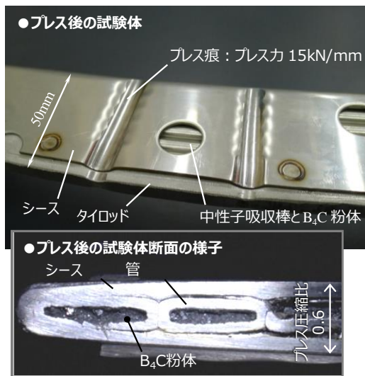
Fig.5 Test piece after press working
