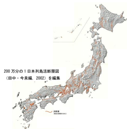
Fig. 3 Distribution of active faults in Japan[4]
