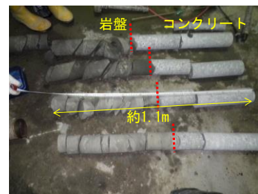
Fig. 6 Cores of low alkaline concrete taken from tunnel support.
