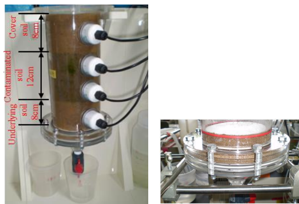
Fig. 3 Columns of the laboratory migration experiments. A column with three soil layers (left) and one with a single contaminated soil layer (right).
