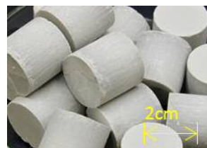
Fig. 5 Pellets made of Kunigel V1 in uniaxial compression using a laboratory-made piston unit.
