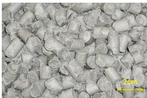
Fig. 9 Cylindrical pellets made by extruding using a 8mm-hole die.
