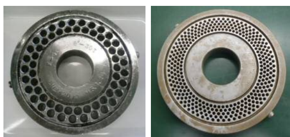
Fig. 8 A die with 8mm holes on the left and another with 3mm holes on the right through which bentonite added water is extruded.
