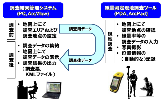
Fig. 1 Schematic procedure and dataflow in the DRaMM-GiGs.
