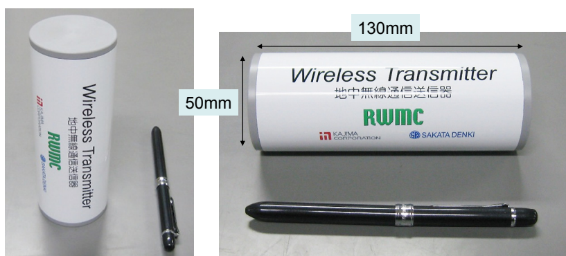
Fig. 11 A miniaturized transmitter of the wireless transmission system in the underground
