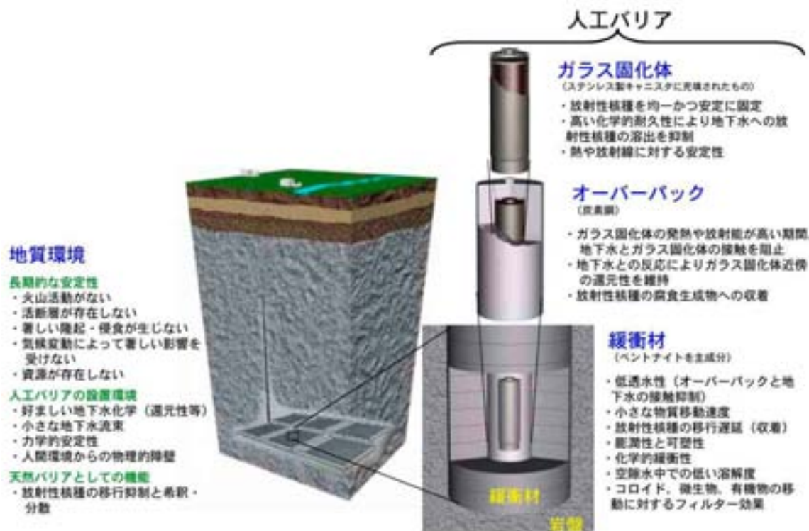
Fig. 1 The set up of the multiple barrier for the geological disposal of HLW [23]
