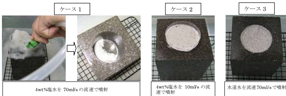
Fig. 14 Appearance of removed bentonite specimen (after 10th flushing)
