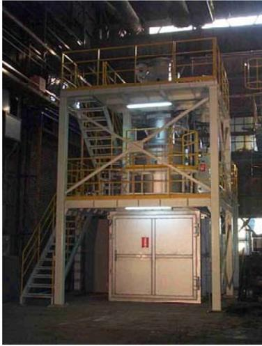
Fig.7 Induction melting system for non-flammable wastes.
