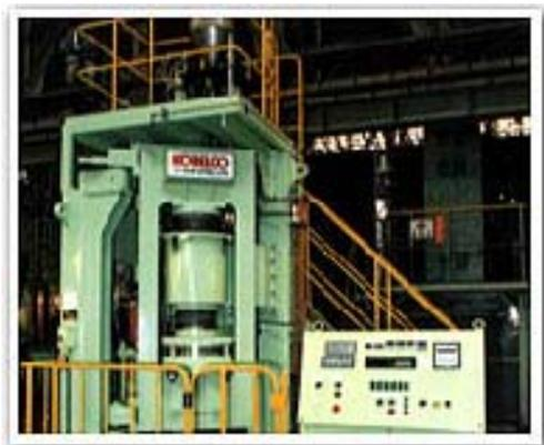
Fig.4 Compression of Hulls and End-pieces.
