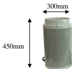
Fig.11 Underground wireless transmission system
