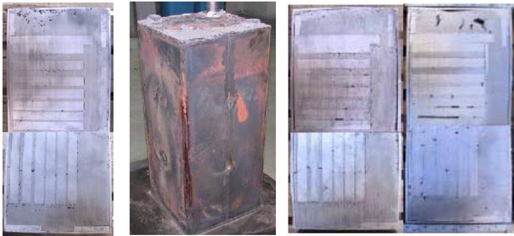
Fig.10 Impurity limit test result Cross section of aluminum impurity test (left), appearance (center), cross section of stainless impurity test (right)
