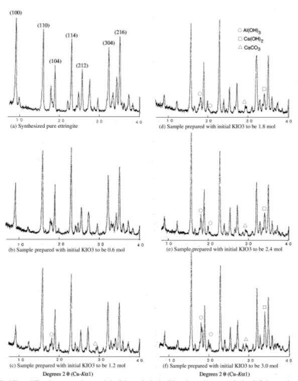
Fig.2 X-ray diffraction pattern characteristic of the synthesized solid products: (a) pure ettringite; (b-f) the samples prepared with initial  $KIO_3$  to be 0.6, 1.2, 1.8, 2.4, and 3.0 mol, respectively.
