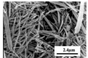
(d) SEM image of sample prepared with initial KIO<sub>3</sub> to be 1.8 mol.
