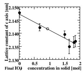
(b) Lattice constant of c axis of synthesized sulfate-iodate ettringite and IO<sub>3</sub> sorbed ettringite.
