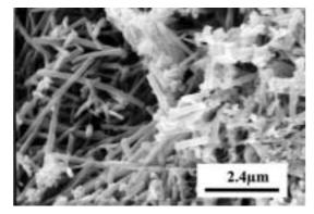
(a) SEM image of sample prepared with no KIO3 reagent
