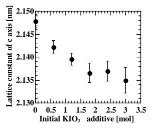
(b) Lattice constant of c axis of synthesized sulfate-iodate ettringite
