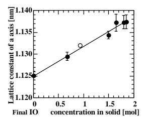
(a) Lattice constant of a axis of synthesized sulfate-iodate ettringite and IO<sub>3</sub> sorbed ettringite.
