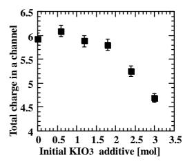
Fig.5 Total charge of anions in a channel of sulfate-iodate ettringite
