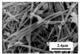
(b) SEM image of sample prepared with initial KIO<sub>3</sub> to be 0.6 mol.
