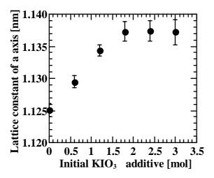
(a) attice constant of a axis of synthesized sulfate-iodate ettringite
