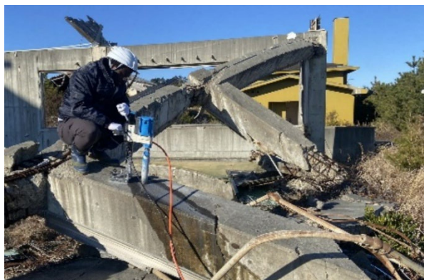
Fig.4 Concrete core sampling
