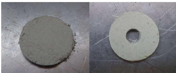
(a) For dielectric constant measurement. (b) For permeability measurement.
