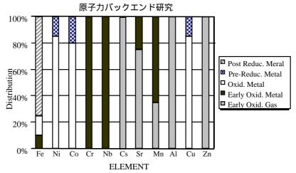
Fig. 14 Small element behavior in oxygen sparging process
