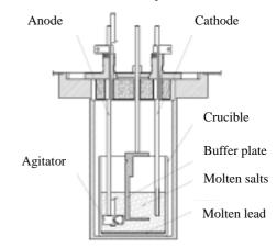
Fig. 11 Schematic drawing of molten salt electro-refining process/ the lead extraction method
