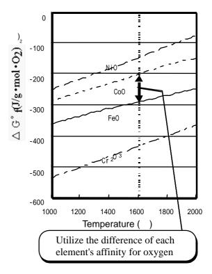
Fig. 5 Principal of oxygen sparging process
