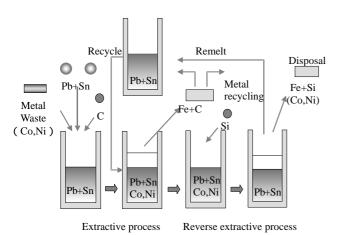
Fig.1 Flow diagram of high temperature extraction process
