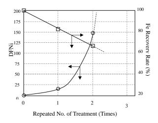
Fig. 4 DFNi, Fe recovery rate and repeated number of high temperature extraction process
