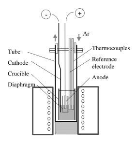
Fig. 10 Schematic drawing of molten salt electro-refining process/ the diaphragm method
