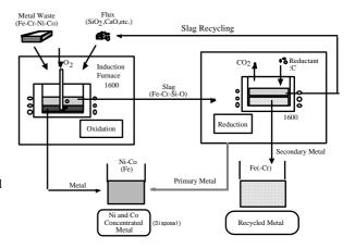
Fig. 6 Concept of oxygen sparging process
