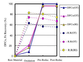
Fig.13 DFCo and Fe recovery rate of oxygen sparging process demonstration tests
