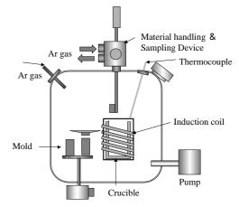
Fig. 2 Schematic drawing of high temperature extraction process
