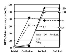
Fig. 8 DFCo, Fe recovery rate of oxygen sparging process screening tests left: carbon steel, right: stainless steel
