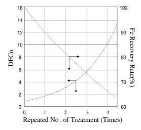
Fig. 3 DFCo, Fe recovery rate and repeated number of high temperature extraction process
