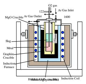
Fig. 7 Schematic drawing of oxygen sparging process
